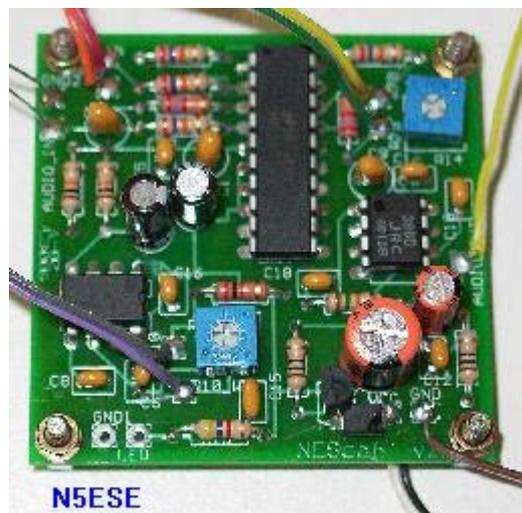
I do wish kit designers would consider putting all I/O components (pots, power connectors, output connectors) on-board, because the bulk of the assembly effort (and time spent, and burned fingers, and wiring errors) come from mounting the controls and wiring them up. Rarely is material cost saved by using panel-mounted controls, but it does take a little extra diligence and forethought during the printed circuit layout stage. Believe me, you'll garner nothing but praise for making the effort.
